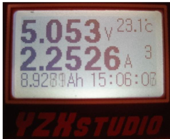
iPad-4 charging at 50% depleted: uses 11.4 watts
