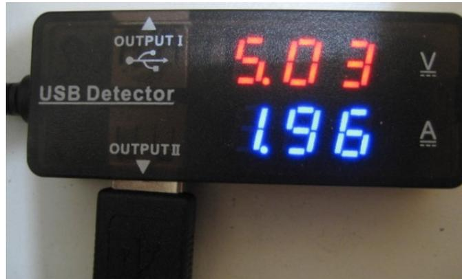
Simple USB meter: voltage and current simultaneously
