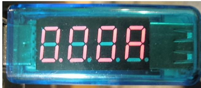
Example above displays voltage and current alternately.
