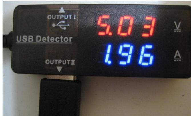
Simple USB meter: voltage and current simultaneously
