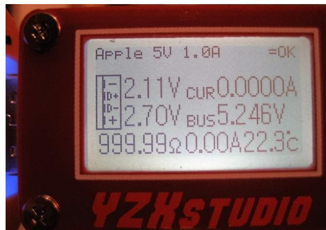
Unit is actually a 1A (5 watt) charger in **both** sockets
