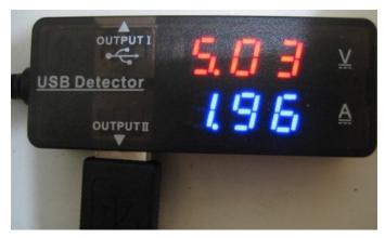
Simple USB meter: voltage and current simultaneously
