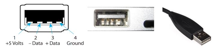
USB Socket Schematic USB-A Socket USB-A Plug
