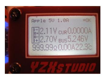
Unit is actually a 1A (5 watt) charger in both sockets
